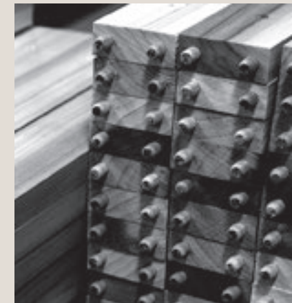
Stronger build process using double dowels and glue
